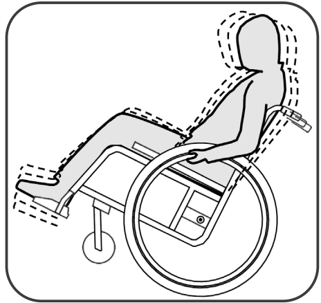
Illustration 30. Finding the critical tipping point of the wheelchair.
