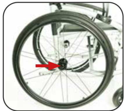
Illustration 10. Attaching or disassembly of wheels.
