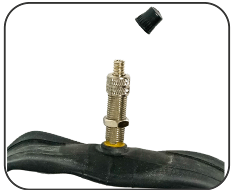
Illustration 13. "Woods" valve (bicycle valve, Dunlop)
