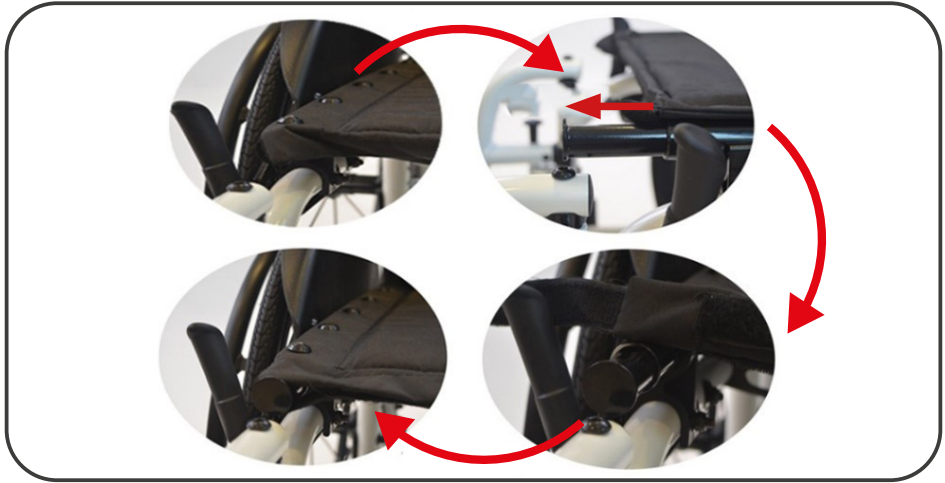
Illustration 17. Seat depth adjustment is available as an option.
